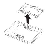
2. Attach the plastic spring to the key board with its flat face downward after confirming the direction.
